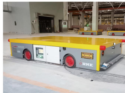
3吨防爆RGV——装备制造 3 tons explosion-proof RGV - Equipment Manufacturing
