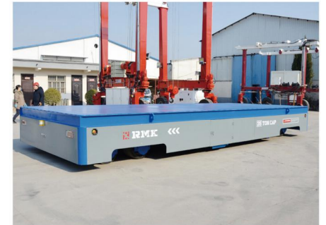
35吨大台面液压转向无轨车——建筑 出口新加坡 35 tons large table hydraulic steering trolley - Buildings Exported to Singapore
